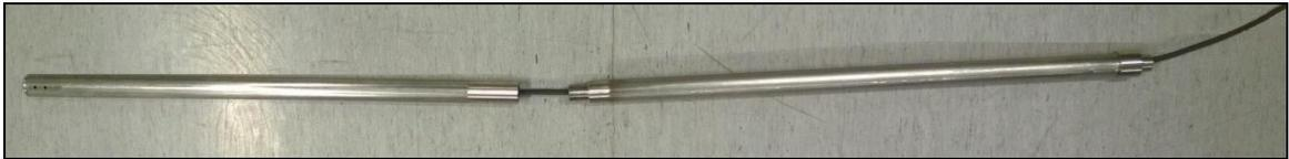
*Fig. 2.5. Optic cable through the second part of sensor head.*
