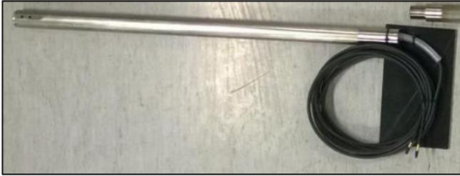
*Fig. 2.4. Sensor head with plastic support and plastic tube.*
