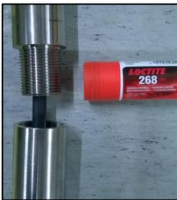
*Fig. 2.6. Threads with Loctite 268.*
