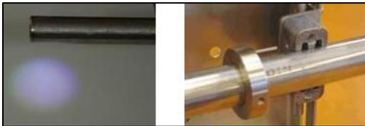
Fig. 5.1. Sensor head light and position memory ring adjustment.
