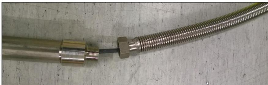
*Fig. 2.7. Fiber optic cable through flexible conduit.*
