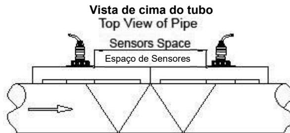
Figure 9: Transducer W Method Mounting
