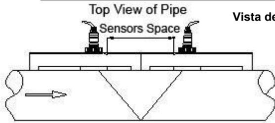
Figure 7: Transducer V Method Mounting
