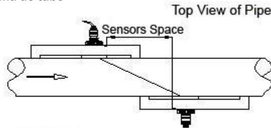
Figure 8: Transducer Z Method Mounting
